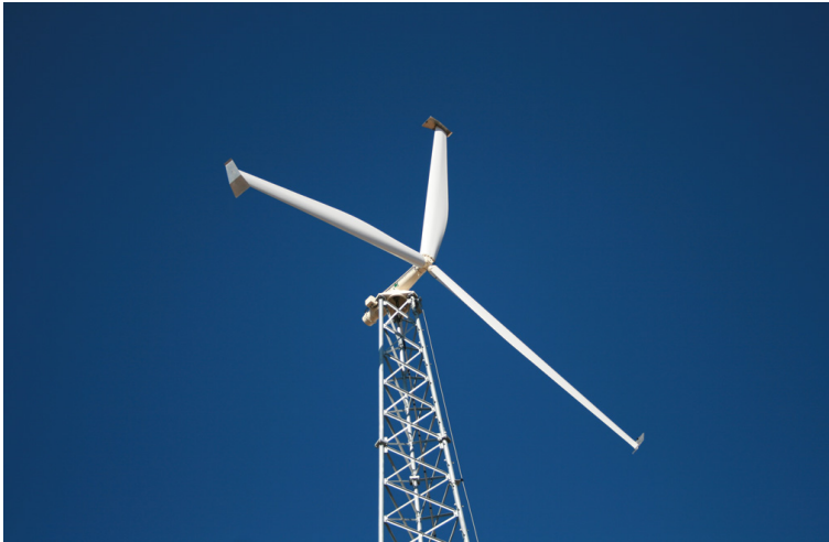
50kW AOC 15/50 wind turbine
