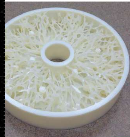
Solomon et al 2014 printed lung phantom containing nodules
