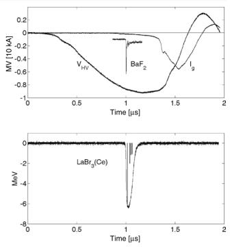
**Figure 5.** A negative 875 kV surge, shown with the current  $I_g$  and x-ray signal (arbitrary units) from an uncalibrated BaF<sub>2</sub> detector alongside the LaBr<sub>3</sub>(Ce) detector. The lower part of the figure shows the signal of the LaBr<sub>3</sub>(Ce) detector and the fitted amplitudes of a train of four pulses.
