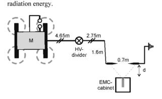
**Figure 1.** Floor plan of the setup, showing the position of Marx generator (M), HV divider, 0.7 m spark gap and EMC cabinet with detector at the distance *d* from the gap.
