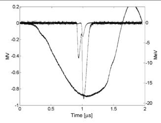
**Figure 7.** Negative surge (left ordinate) and x-ray signals (right ordinate) seen by two detectors, one without (large signal) and one with (smaller signal) a 1.5 mm Pb absorber.
