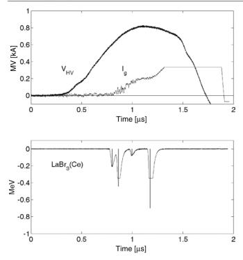
**Figure 4.** Positive surge with 810 kV maximum, shown with the current  $I_g$  during the leader initiation phase. At 1.5  $\mu$ s the gap breaks down. Four x-ray pulses can be distinguished. The  $\gamma$ -detector and current signals are clipped by the oscilloscope. The vertical bars indicate the maximum equivalent energy and its timing obtained by the fit.
