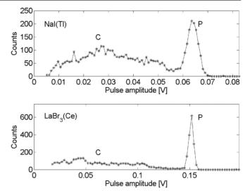
**Figure 2.** <sup>137</sup>Cs pulse height spectrum for NaI(Tl) and LaBr3(Ce) detectors of 5000 pulses recorded by an 8 bit resolution oscilloscope. The horizontal axes have been scaled to coincide on the photopeak.
