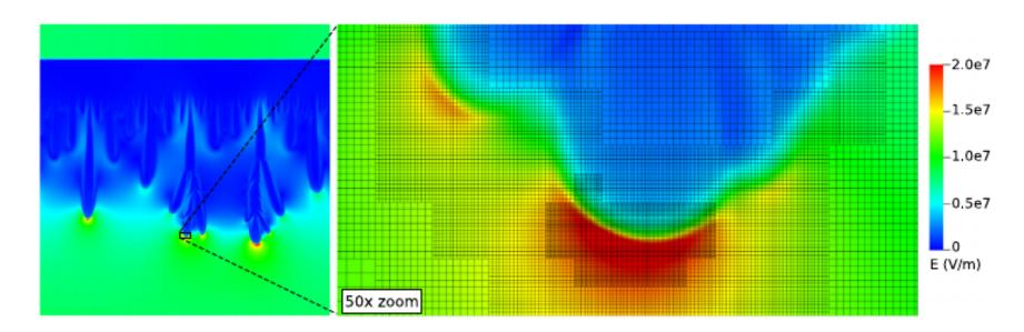
**Fig. 9.** The full domain and a 50 times zoom, which shows the electric field and the mesh around a streamer head at t=8 ns. The finest grid spacing is  $\Delta x \approx 1.22$  m.
