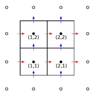
**Fig. 2.** Location and indices of the cell-centered variables (black dots) and the face-centered variables in the x-direction (horizontal arrows) and y-direction (vertical arrows) for a box of 2  $\times$  2 cells. The ghost cells for the cell-centered variables are shown as circles.
