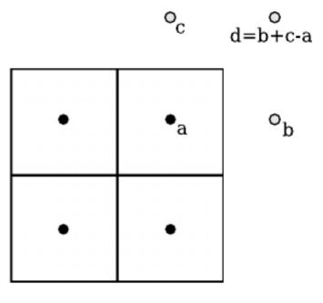
**Fig. 3.** Illustration of the linear extrapolation procedure for corner ghost cells in 2D that is used when the diagonal neighbor is missing. The corner ghost cell gets a value b + c - a.
