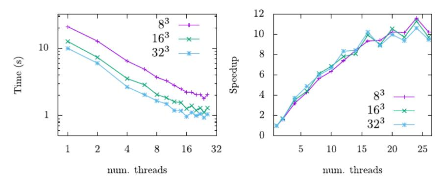
**Fig. 7.** Duration (left) and speedup (right) of a single FMG cycle on a uniformly refined grid of 512  $^3 \approx 134 \times 10^6$  cells versus the number of OpenMP threads. Results are shown for octrees with boxes of 8  $^3$ , 16  $^3$  and 32  $^3$  cells.
