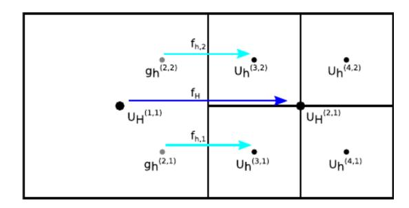
**Fig. 5.** Illustration of a refinement boundary. The cell centers are indicated by dots. There are two ghost values (gray dots) on the left of the refinement boundary. Fluxes across the refinement boundary are indicated by arrows.
