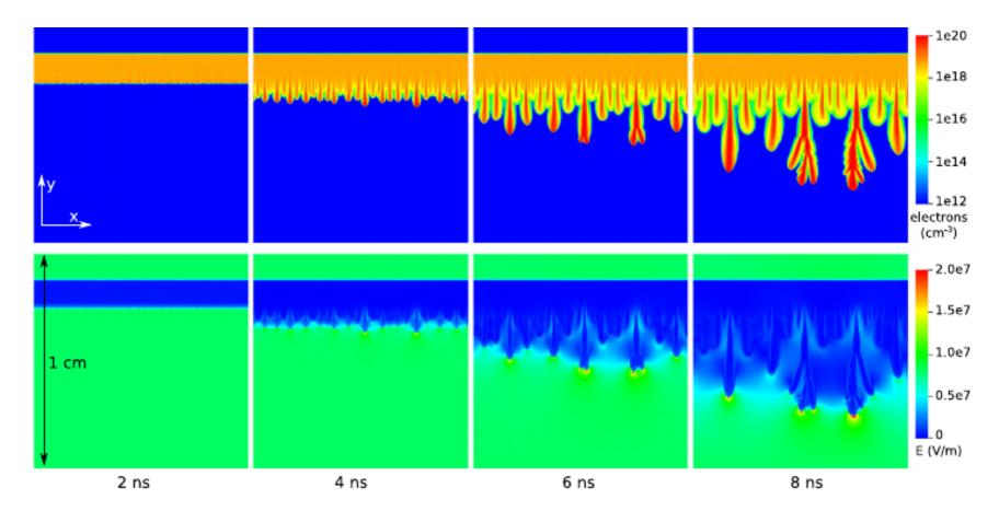
**Fig. 8.** The evolution of the electron density (top) and electric field (bottom) in a 2D electric discharge simulation in nitrogen at standard temperature and pressure. The discharge started from a pre-ionized layer, which destabilizes into streamer channels. A zoom-in of the mesh around a streamer head at t = 8 ns is shown in Fig. 9.
