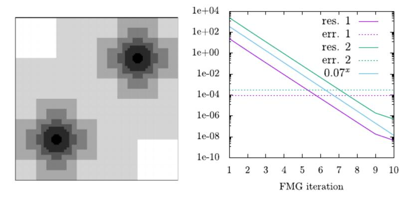
**Fig. 6.** Left: mesh spacing used for the multigrid examples, in a  $[0, 1] \times [0, 1]$  domain. Black indicates  $\Delta x = 2^{-11}$  and white  $\Delta x = 2^{-5}$ . Right: the maximum residual and maximum error versus FMG iteration. Case 1 corresponds to a standard Laplacian (Eq. (9)) and case 2 to the cylindrical case with a jump in  $\varepsilon$  (Eq. (10)).
