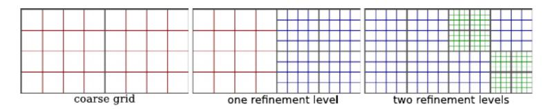
**Fig. 1.** Left: example of a coarse grid consisting of two boxes of 4 × 4 cells. The middle and right figure show how the boxes can be refined, by covering them with four 'child' boxes.
