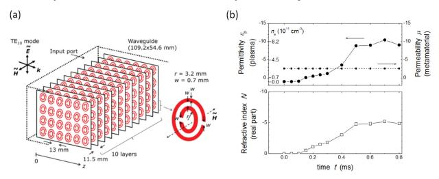
**Figure 4.** (a) Schematic of magnetically-active metamaterial that is inserted into an argon-filled waveguide section in which plasma is formed by pulsed excitation. (b) Time-variation in the measured dielectric constant and corresponding refractive index within the metamaterial-filled section. Note transition to negative values due to plasma density evolution to above cut-off values.
