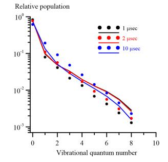
**Figure 26.** Population of vibrational levels in  $N_2$  measured by ps-CARS in a pin-to-pin discharge at 133 hPa. Reproduced from [139]. © IOP Publishing Ltd. All rights reserved.
