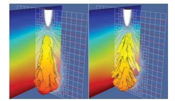
**Figure 32.** Particle in cell simulation of breakdown in 100 Torr of argon for point-to plane potential of (left) 3.25 kV and (right) 5 kV using AMR techniques. Isosurfaces of electron density ( $10^{16} \text{ m}^{-3}$  and  $5 \times 10^{16} \text{ m}^{-3}$ ), adapted grids, and equipotential lines are shown. Reproduced from [164]. © IOP Publishing Ltd. CC BY 3.0.
