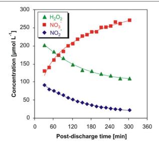
**Figure 27.** Post-discharge evolution of  $H_2O_2$ ,  $NO_2^-$  and  $NO_3^-$  in aqueous solution (pH 3.3) after treatment by the air discharge plasma. Reproduced from [140]. © IOP Publishing Ltd. All rights reserved.
