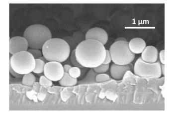
**Figure 12.** Core–shell nanocapsules produced in an aerosolassisted AP PE-CVD process. The shell is made of a hydrocarbon membrane originated from the ethylene feed in the discharge. The core contains a droplet of a biomolecule solution.
