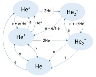
**Figure 35.** Illustration of a simplified mechanism in helium. A rate must be associated with each arrow to fully define the mechanism.
