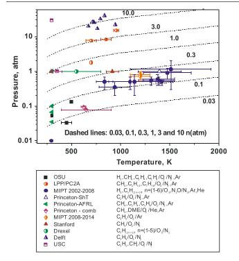
**Figure 21.** *P*–*T* diagram [113] of results available in the literature from experiments on combustion initiated or assisted by nanosecond discharges. Dashed lines are the isolines of the gas density, normalized with respect to the atmospheric gas density  $n_{\text{atm}}$  for normal conditions. Reproduced from [113]. © IOP Publishing Ltd. All rights reserved.
