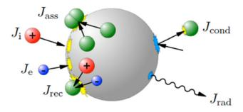
**Figure 13.** Schematic of the energy exchanges between nanoparticles and the surrounding plasma. Nanoparticles receive energy through energetic surface reactions, such as electron and ion bombardment, recombination, and association reactions. They lose energy through conduction to the neutral gas and radiation. Reproduced from [74]. © IOP Publishing Ltd. All rights reserved.
