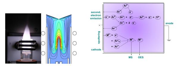
**Figure 28.** Left: photograph of argon ICP used for elemental and metallomics analysis by either emission or mass spectrometry. Center: calculated sample ion density profile (color contours) and plasma temperature profile (black contour lines) in the ICP. Right: schematic diagram of the most important mechanisms in a moderate-pressure GD, used for bulk and depth-resolved analysis of solid samples.
