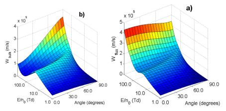
**Figure 7.** Multi-term solutions of the Boltzmann equation for drift velocities (a) bulk and (b) flux for positrons in CF<sub>4</sub> in combined electric and magnetic fields for  $B/n_0 = 1000$  Hx, (in units Huxley, 1 Hx =  $10^{-27}$  Tm<sup>3</sup>,  $n_0$  is the gas number density) as a function of  $E/n_0$  (in units Townsend 1 Td =  $10^{-21}$  Vm<sup>2</sup>) and the angle between the two fields.
