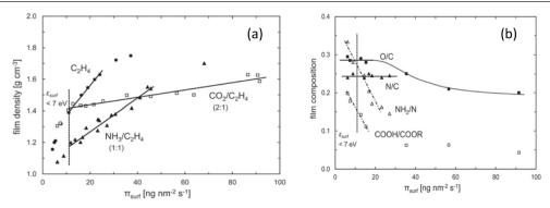
**Figure 9.** Comparison of film density (a) and functional group density (b) for plasma-based deposition of plasma-polymer films versus momentum transfer to the surface during deposition. Reprinted from [53], with the permission of AIP Publishing.
