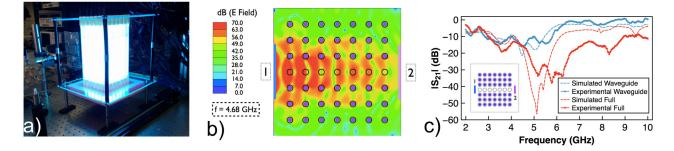
**Figure 3.** (a) Photograph of a plasma photonic crystal array comprised of  $7 \times 7$  high current density discharge tubes. (b) Simulated waveguide performance when a row of the discharges is turned off and an antenna is placed at location 1, to transmit an EM wave to location 2. (c) Comparison of measured and simulated transmission ( $S_{21}$ ) spectra for the configuration in (b).
