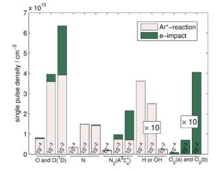
**Figure 16.** Results from a model of a shielded Ar kinpen device at atmospheric pressure with predictions of RONS densities generated by a single guided streamer at dry synthetic air mole fractions  $10^{-4}$ ,  $10^{-3}$  and  $10^{-2}$ . Contributions from direct electron impact reactions and reactions involving excited argon species are distinguished: note the importance of Ar metastables as reactive precursors in this study. Reproduced from [88]. © IOP Publishing Ltd. All rights reserved.
