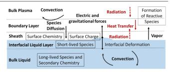
**Figure 5.** Schematic representation of the key plasma–liquid interactions. The boundary layer reflects the gradients in temperature, species densities and gas flow velocities. The sheath is present for ionizing plasmas when the liquid surface is charged.
