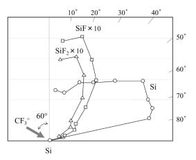
**Figure 10.** Angular distributions of desorbed species when a single crystal Si (100) surface is exposed to a  $500 \text{ eV } \text{CF}_3^+$  beam at an incident angle of  $60^\circ$ . The radius of the polar graph (i.e. the distance between the origin and a point on the curve) is proportional to the flux of desorbed species. Reproduced from [56]. © IOP Publishing Ltd. All rights reserved.
