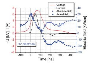
**Figure 8.** Electric field in quasi-2D ns pulse discharge 'curtain' plasma in ambient air, measured by ps 4-wave mixing ~100  $\mu$ m from the high-voltage electrode. The discharge is sustained between a steel razor blade and grounded copper foil covered by a quartz plate with a thickness of 120  $\mu$ m. The discharge gap is 600  $\mu$ m. Reproduced from [45]. © IOP Publishing Ltd. All rights reserved.
