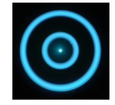
**Figure 22.** Front view of the 10 kW class X2 two-channel nested Hall thruster with its centered-mounted cathode firing with xenon at full power in dual channel configuration. Image courtesy of Ray Liang, reproduced with permission.
