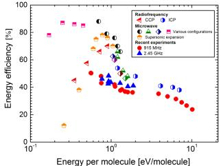
**Figure 20.** The energy efficiency of  $CO_2$  dissociation for various plasma reactors (CCP capacitively coupled plasma, ICP inductively coupled plasma and microwave plasmas (flow and supersonic expansion)). Data taken from [106, 107] with recent results from the DIFFER institute using flowing microwave reactors.
