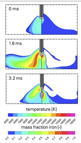
**Figure 24.** Calculated distributions of arc temperature (left) and iron vapour mass fraction (right) at different times in pulsed metal-inert-gas welding of iron. The arc current at the successive times is 50, 420 and 150 A, respectively. The changes in location of the iron vapour production as the arc current changes lead to changes in the distribution of current density and temperature in the arc. Springer [125] © International Institute of Welding 2016, with permission of Springer.
