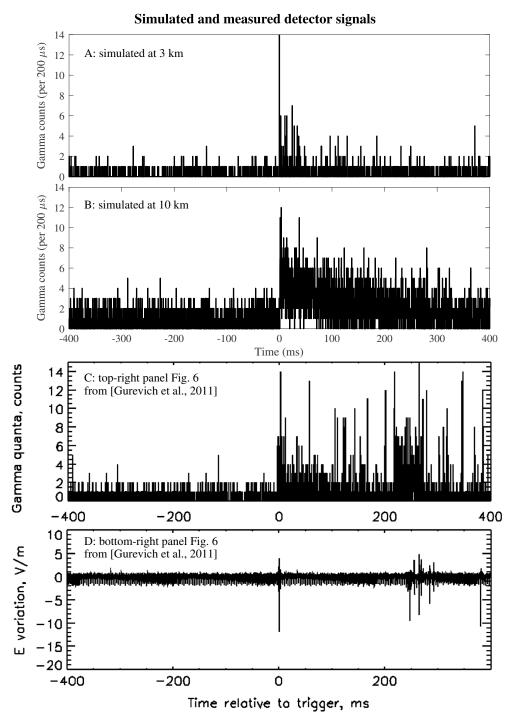
**Figure 4.** (a, b) Simulated counts of gamma radiation from the simulation presented in Figures 2 and 3. (c, d) Taken from Gurevich et al. (2011), in which it is denoted there as event "6." Figures 4a to 4c are gamma ray counts per 200  $\mu$ s interval on a detector of 475 cm<sup>2</sup>, at 3, 10, and 3.8 km, respectively. Figure 4d gives the measured fast electric field variation (20  $\mu$ s sampling rate measured by the capacity sensor, see Gurevich et al., 2011 for more details).
