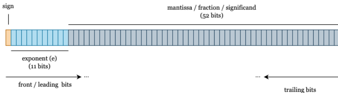
Figure 2.7: IEEE 754 double precision floating-point bitwise representation. One bit for sign, 11 bits for exponent and 52 bits for mantissa / fraction.
