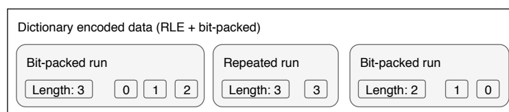
FIGURE 2.12: Example of RLE_DICTIONARY encoded data in Parquet, bit-packed and RLE runs are mixed
