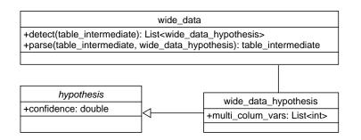
FIGURE B.7: Wide Data Class Diagram
