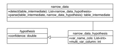
FIGURE B.8: Narrow Data Class Diagram
