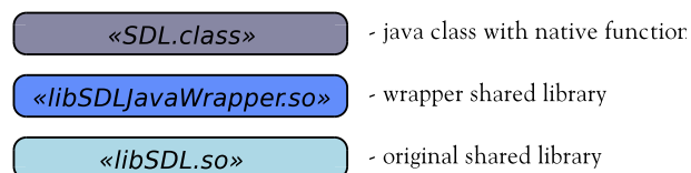
Figure 5.1: Interfacing to existing libraries: The Java Native Interface requires an extra wrapper library.
